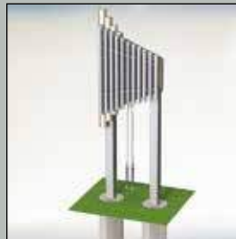
Steel Post In-Ground
